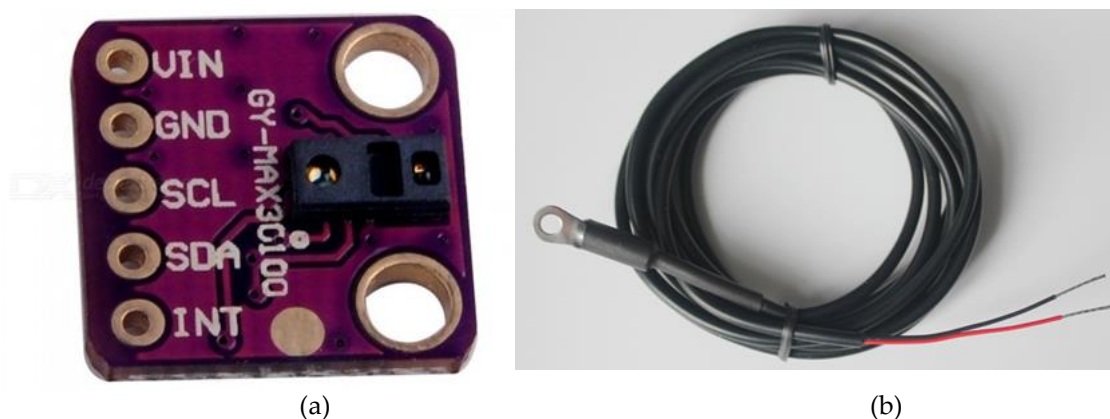
Figure 2. Sensor Modules for Arduino Based PM3P (a) MAX30100 [9] (b) DS18B20 lug type [10]
