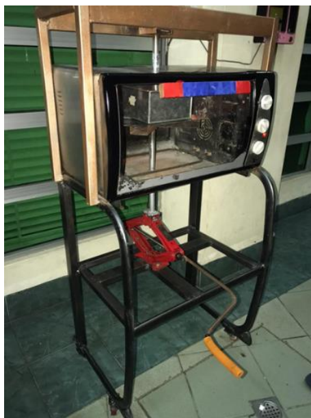
Figure 5. The fabricated Plastic Compressor Machine
