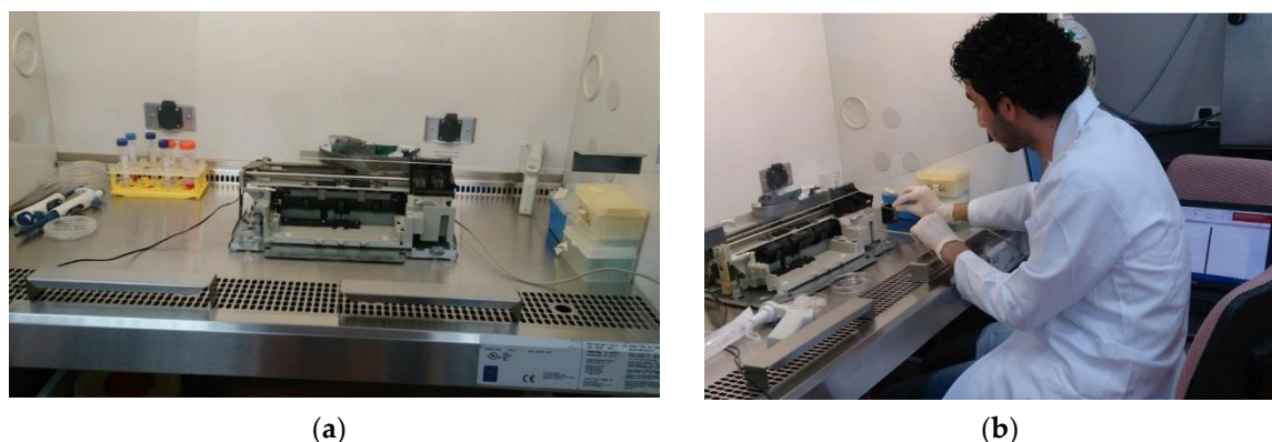
Figure 1. Modification process of (a) modified regular printer into Bioprinting; (b) Testing of the 3D Bioprinting
