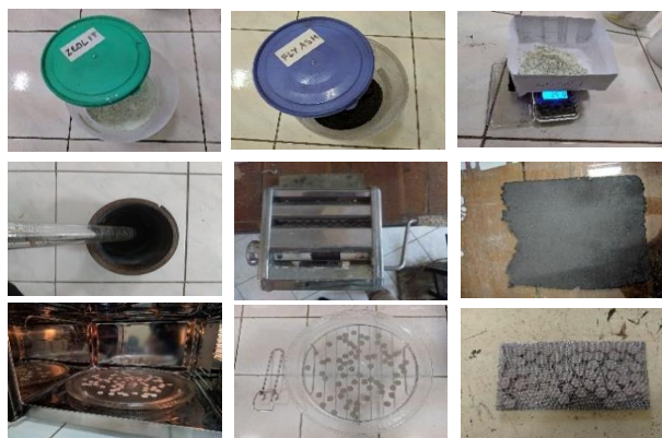
Figure 1. Manufacturing process of zeolite-flyash filter
