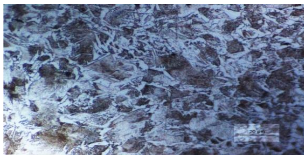
Figure 7. Microstructure of AISI 1020 steel quenching oil media 500x magnification.
