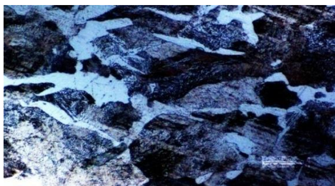
Figure 5. Microstructure of AISI 1020 steel raw material magnification 500x
