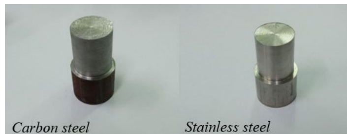
Figure 9. The results of the turning machining for carbon steel and stainless steel materials
