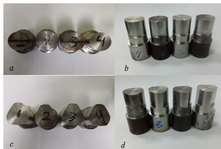
Figure 10. Final results of profiling P2 and PC3; (a) top view of P2 profiling results; (b) side view of P2 profiling results; (c) top view of PC3 profiling results; and (d) side view of PC3 profiling results
