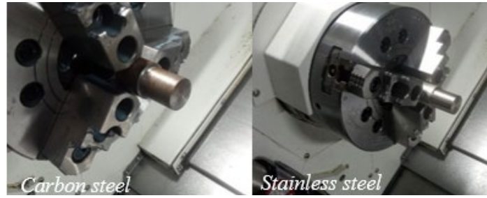
Figure 7. The results of the roughing process of carbon steel and stainless steel materials
