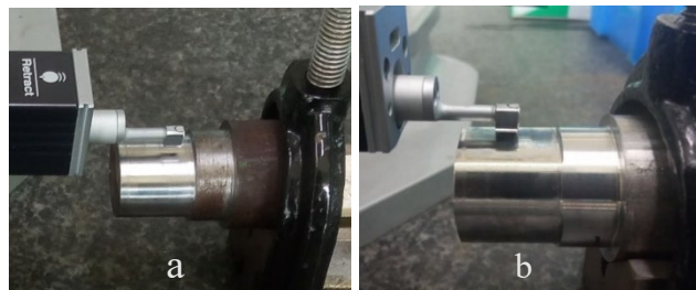
Figure 2. Roughness measurement of shaft profile (a) P2; (b) PC3
