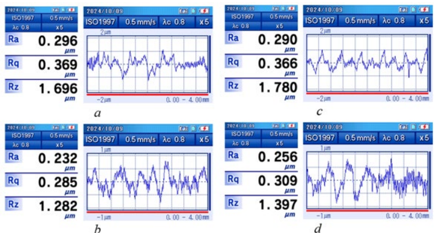
Figure 11. The results of measuring the surface roughness of the PC3 profile on one side of each test, (a) carbon steel with DoC 0.2 (b) stainless steel with DoC 0.2 (c) carbon steel with DoC 0.3 (d) stainless steel with DoC 0.3
